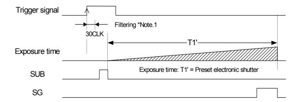
Notes: The trigger signal equal to or shorter than 30 CLK is removed by the filtering system. Input trigger signal has to be more than 31 CLK pulse width.
